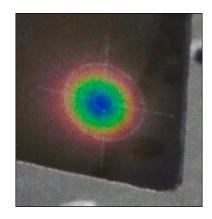
crystals can be calibrated to precise temperature values and therefore also make excellent thermometers. Leuco dyes, while operating in a much wider range of temperatures, have less accurate temperature response. These are a good indicator of whether the object is either "hotter than", "colder than", or "just about" the threshold temperature. As these are relatively inexpensive, these find applications in security printing, toys, battery testers, smart packaging, and such.
